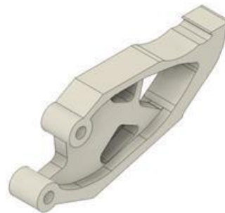
Figure 6. Design view with 40% mesh optimization
